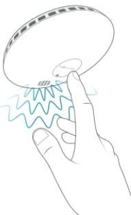
**EN** You should test the smoke detector every month to ensure that it is properly installed and working correctly. You can carry out the test directly on the detector by pressing the central button for three seconds.
