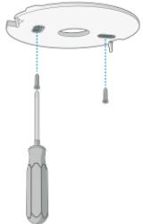
**EN** Fix the plate to the ceiling using the screws provided.
